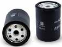
AFF6013 A: 77 B: 72 C: 116 D: M16 X 1.5 OEM : 142139393 MANN: WK731 VOLVO -BUDSUN
